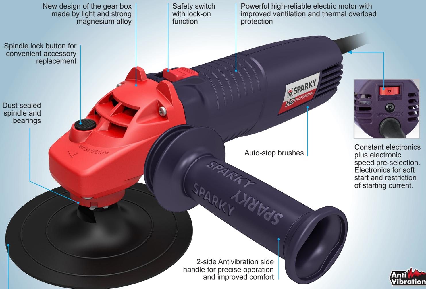
Flexible backing pad Ø148 mm for hook and loop accessories
