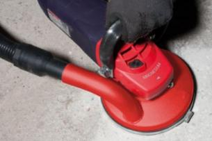
compliant anti-burst and anti-rotation blade guards to further protect the user.
